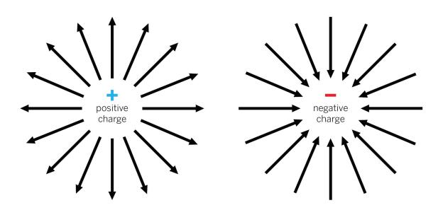
There are two kinds of electric charge: positive and negative. In a diagram of an electrostatic field, the arrows show the direction of the force that would be exerted on a positive charge.
